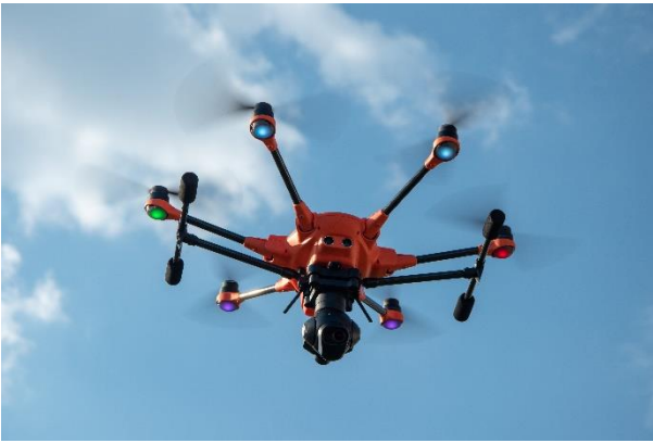
Fig. 5. Drone carrying thermal camera
